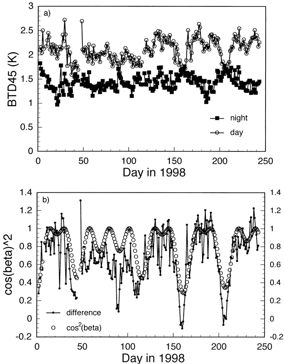
FIG. 10. Variation of (a) mean daily brightness temperature difference between VIRS channels 4 and 5 for  $T_4 < 240$  K and (b) the day–night differences in  $BTD_{45}$  and the squared cosine of the TRMM beta angle.
