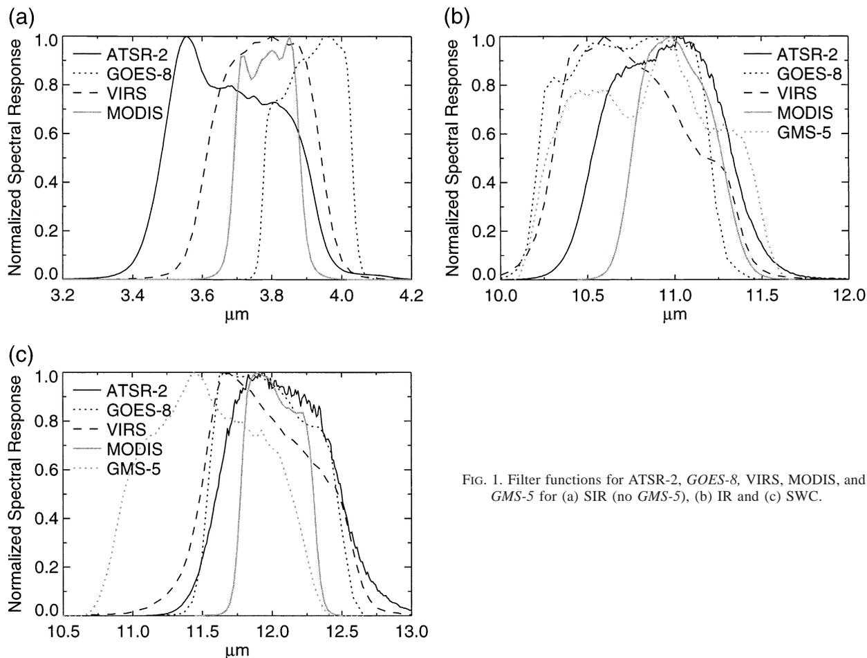
FIG. 1. Filter functions for ATSR-2, *GOES-8*, *VIRS*, *MODIS*, and *GMS-5* for (a) SIR (no *GMS-5*), (b) IR and (c) SWC.
